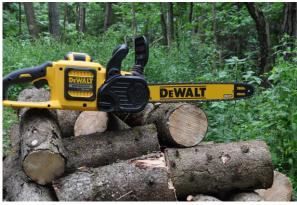
a variable speed trigger switch. You must continue to squeeze the trigger to keep the saw running. The 16" Oregon bar and chain is another nice feature. The charger is easy-to-use and the battery features a fuel gauge.
